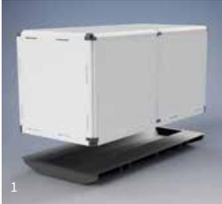
In order to meet our structure-borne noise requirements we designed a new base frame concept (1). Through FEA and specific mount selection (both single and double) an optimal result can be achieved.
